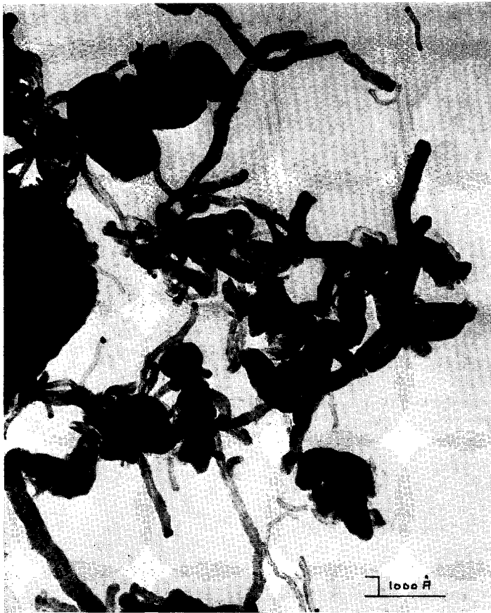
FIG. 2. Electron micrograph of whisker-like carbon formed by decomposition of \text{CH}_4 on catalyst B1 at 500^\circ\text{C} .
